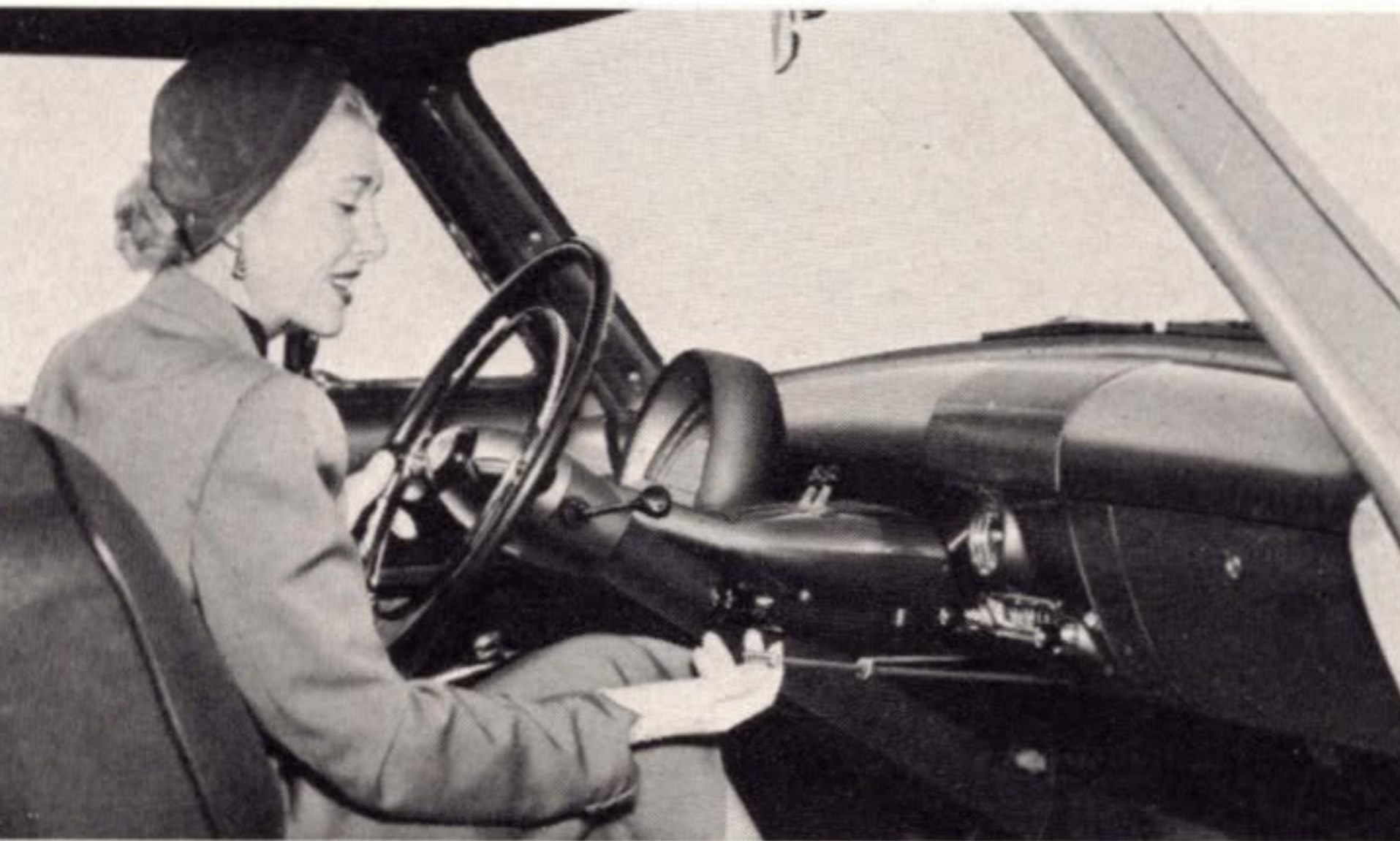
Handy control handle permits Overdrive to be locked "in" or "out."
