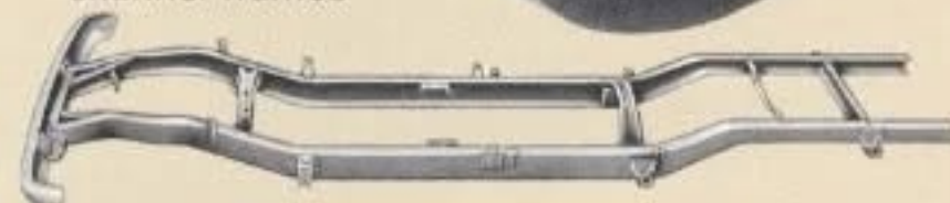
True truck type assure stamina and rigidity. Drop section protects between-axle parts, puts cab at low height.
