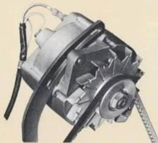
standard 37-amp, alternator —Better than a generator, supplies charging current at engine idle, thus reduces load imposed upon the battery, lengthens battery life. Is also itself longer-lived and simpler to service.
