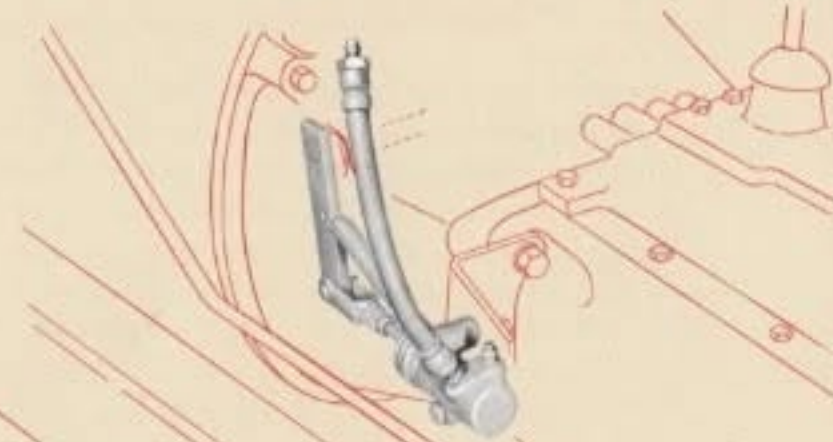
clutch hydraulic control —Reduced pedal effort, less linkage maintenance are benefits of this control for all clutches from 10-in. 6-spring to 12-in. 12-spring.
