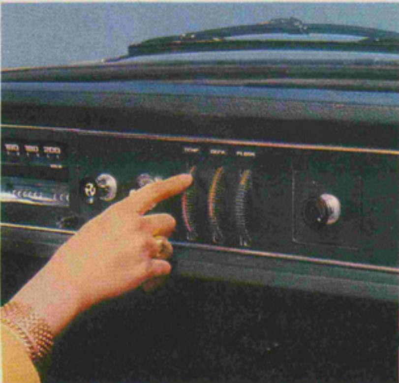
Three vertically mounted discs recessed into the dashboard control the volume, temperature and distribution of air. A fingertip is all that's required to operate these discs which have illuminated strips for easy identification at night. So day or night you can tell at a glance just how much warm air is going where.
